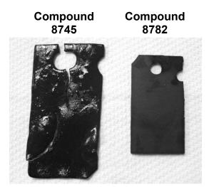
ASTM D 471 Volume Swell sample after aging 480 hours @ 250° F . (Samples shown 3/4 size)
